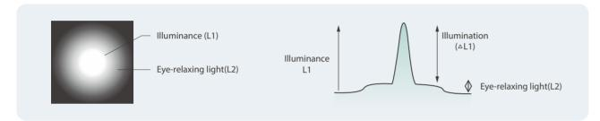
The Illuminating Engineering Society of North America (IESNA) describes reducing contrast between the surgical site and peripheral region improve relaxing and visual performance. Ratios in excess of 40:1 can be suitable, but this ratio should be minimized wherever possible.
